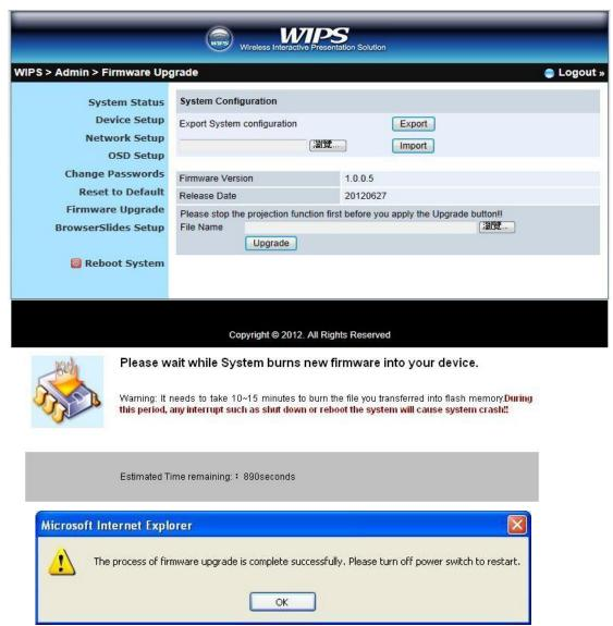
**Warning:** Don't power off WIPS TWP-1000 while firmware upgrade in progress, otherwise will cause your Box doesn't work and have to return device to your vendor for fixing.
