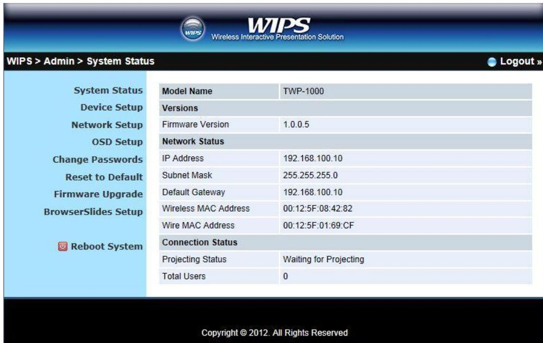
The screenshot shows the WIPS Admin interface. The breadcrumb navigation is 'WIPS > Admin > System Status'. A 'Logout' button is in the top right. On the left is a navigation menu with options: System Status, Device Setup, Network Setup, OSD Setup, Change Passwords, Reset to Default, Firmware Upgrade, BrowserSlides Setup, and Reboot System. The main content area displays system information in a table format:
